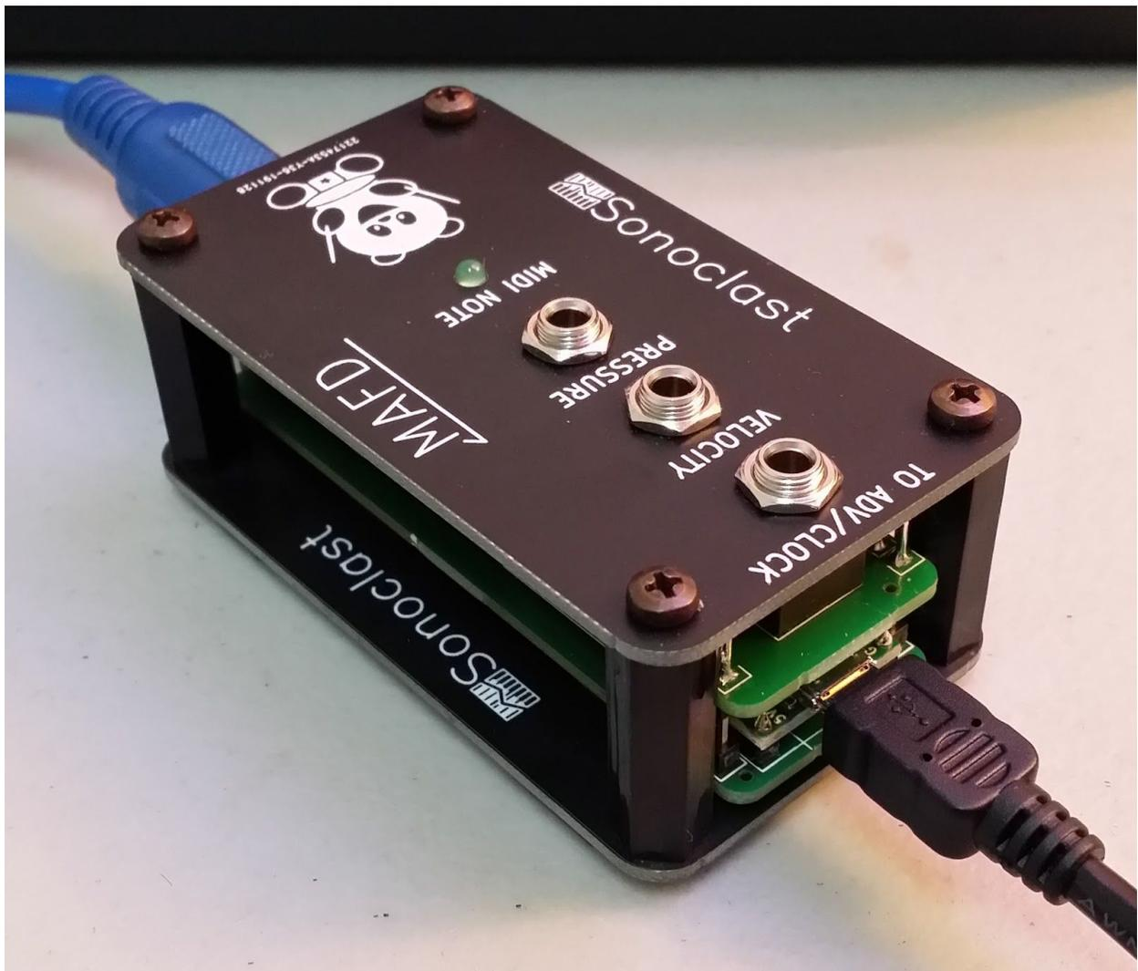
2. Use the USB cable for MIDI (plugged into your computer), or connect a MIDI DIN cable from the MIDI OUT of your controller to the DIN connector on the MAFD.
